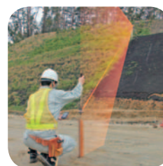
Instrument at any given point and measure 2 points (coordinate origin and a point on one of coordinate axis)
