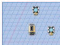
Resection (Instrument at any given point and measure 2 known points)
