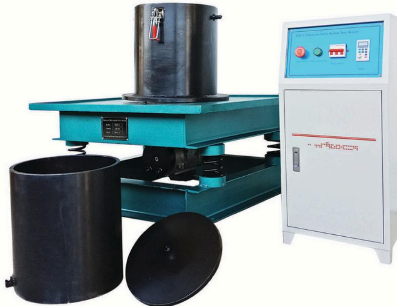
**Standard :** ASTM D4253/D4254, pr EN 13286-5
