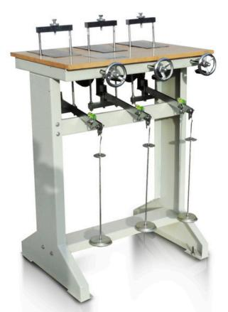
**For lower press:** The testing sample area is 30cm square, press range is 12.5Kpa to 800Kpa. The testing sample area is 50cm square, press range is 12.5Kpa to 400Kpa.
