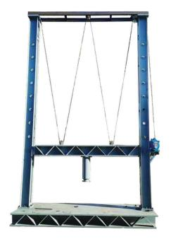
The Concrete pipe testing machines are consisting of a frame and a hydraulic power pack. The frames are rigid 2 column constructions with superior axial and lateral stiffness and are precision aligned. Integrated in the crosshead is a double acting actuator in servo-quality. The actuator has anti-rotation system to prevent the natural tendency of the actuator to rotate. The stroke of the double acting actuator is 300 mm. Load cell is used for precise load measurement and closed loop control.
