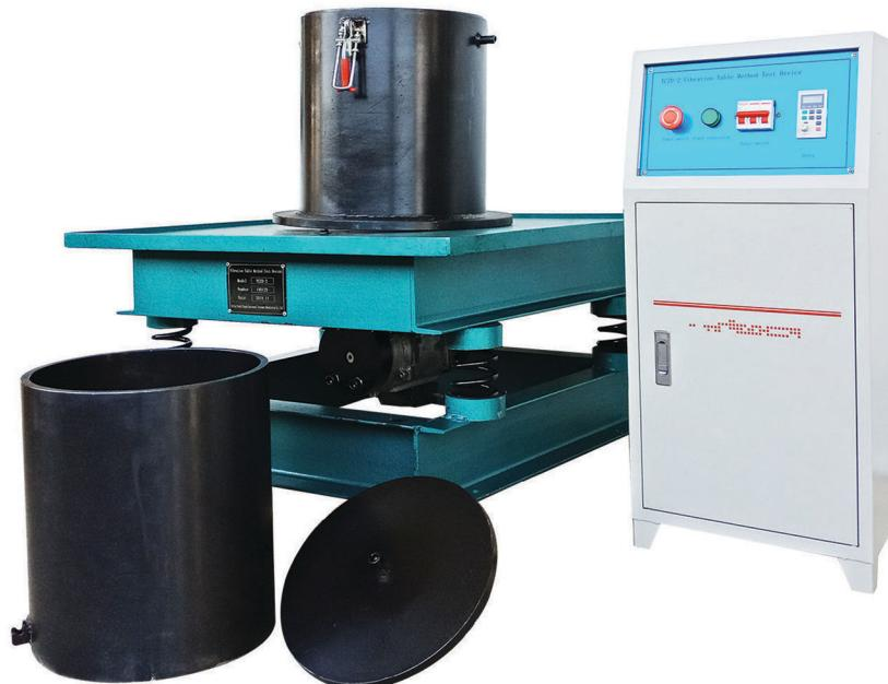
**Standard :** ASTM D4253/D4254, pr EN 13286-5
